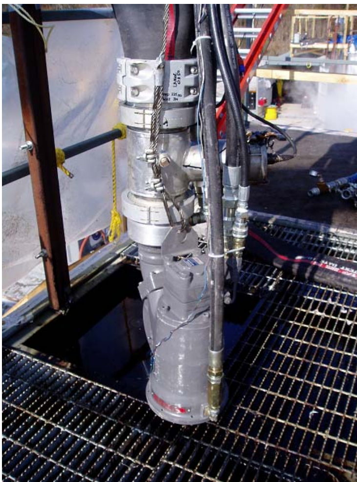
Figure 63 LAMOR GT-A 50 ready for Deployment. Note the compact and sleek overall concept with the fewest possible protruding parts and simple hose arrangement.
