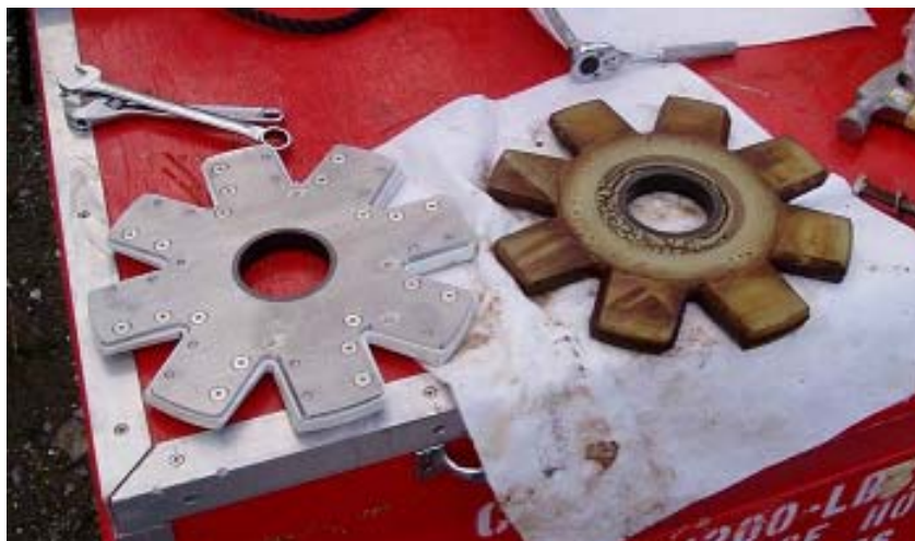
Figure 64 GT-185 High Pressure/High Temperature Plate Wheel (Left) GT-185 Standard Plate Wheel (Right)
