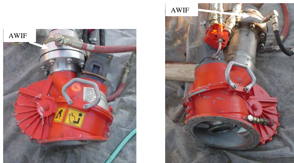
Figure 46 US Navy DOP-250 with "new" flemingCo discharge side AWIF (left) USCG DOP-250 with "old" USN/USCG/FRAMO type discharge side AWIF (right)
