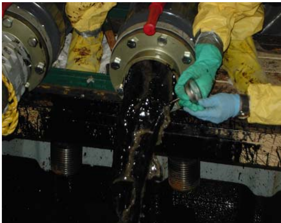
Figure 51 Oil and lube water discharge in Test 3 with USCG DOP-250 pump, with flemingCo Inlet AWIF and USCG/USN Outlet AWIF, 185,000 cSt test oil through 1514.5 ft. hose. Note the oily lube water.
