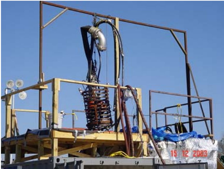
Figure 58 CCG GT-185 w. USN Steam Coils for DOP-250 and riser hose ready for deployment over the USCG Test Tank
