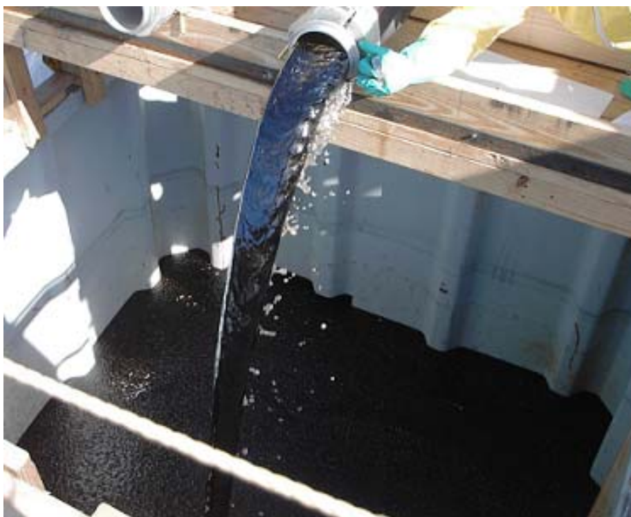
Figure 48 Oil and Lube Water Discharge in Test 0/1 with USCG DOP-250 w. USCG/USN Outlet AWIF on 21,000 cSt Oil and 107.5 ft Hose
